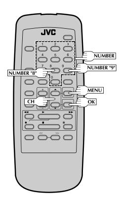
You can directly program the VCR's timer to record up to 8 shows, as far as a year in advance. Remember, the clock must be set before you can program the timer (127 pg. 8).
